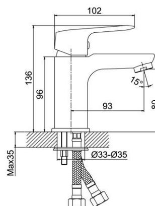
**ESPECIFICAÇÕES | SPECIFICATIONS****PT****Cartucho de discos cerâmicos BRUMA****SmoothBreeze®****Ligações flexíveis****Sistema de poupança de água BRUMA EcoDrop®****EN****Ceramic cartridge BRUMA SmoothBreeze®****Flexible connection hoses****Water-saving technology BRUMA EcoDrop®****DIAGRAMA DE CAUDAL | FLOW DIAGRAM**
