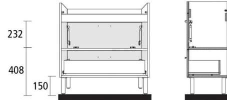
**DIMENSÕES | DIMENSIONS** 810mm (L) x 810mm (A) x 360mm (P)
