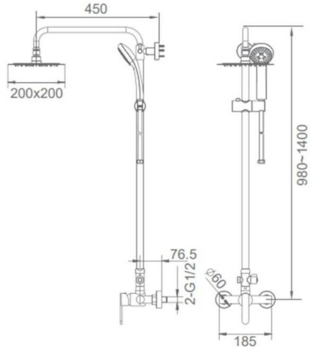
**DIMENSÕES | DIMENSIONS** 450mm (C) x 185mm (L) x 1300mm (A)
