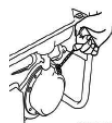
Align the notch on the starter pulley with the hole at the top of each starter.
