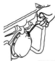
Align the catch on the starter pulley with the hole at the top of recoil starter.
