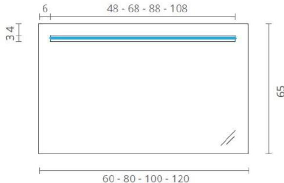
**DIMENSÕES | DIMENSIONS** 600mm (L) x 650mm (A) x 4mm (P)
