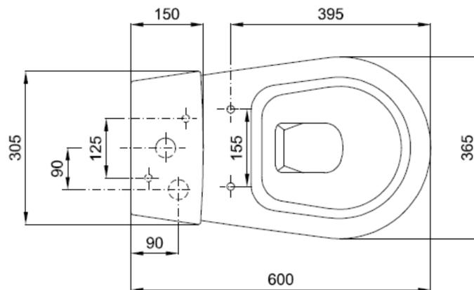
**DIMENSÕES | DIMENSIONS** 365mm (C) x 600mm (L) x 395mm (A)
