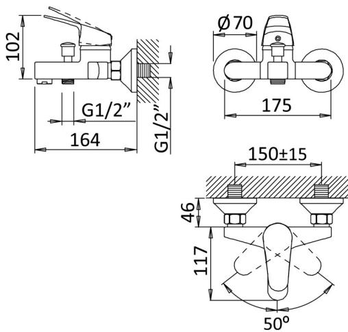
**DIMENSÕES | DIMENSIONS** 175mm (C) x 150mm (L) x 102mm (A)
