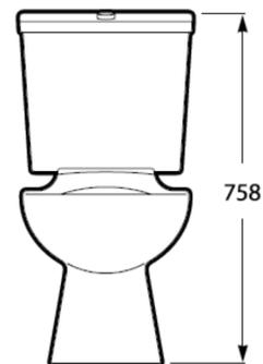
**DIMENSÕES | DIMENSIONS** 375mm (C) x 438mm (L) x 758mm (A)
