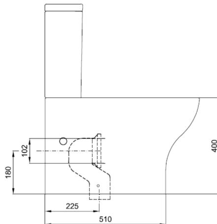
**DIMENSÕES | DIMENSIONS** 345mm (C) x 625mm (L) x 395mm (A)
