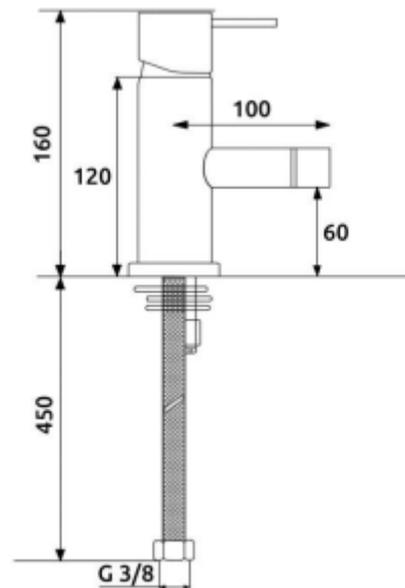
**DIMENSÕES | DIMENSIONS** 100mm (C) x 35mm (L) x 160mm (A)
