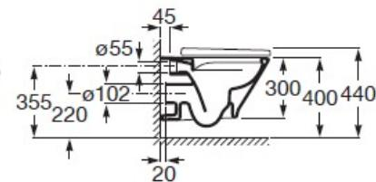
**DIMENSÕES | DIMENSIONS** 355mm (C) x 540mm (L) x 440mm (A)
