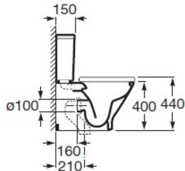
**DIMENSÕES | DIMENSIONS** 365mm (C) x 600mm (L) x 790mm (A)
